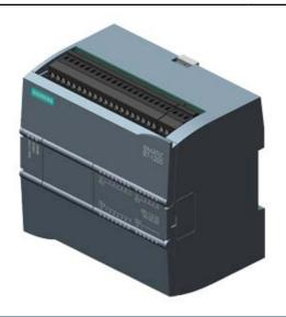
SIMATIC S7-1200, CPU 1214C, COMPACT CPU, DC/DC/DC, ONBOARD I/O: 14 DI 24V DC; 10 DO 24 V DC; 2 AI 0 - 10V DC, POWER SUPPLY: DC 20.4 - 28.8 V DC, PROGRAM/DATA
